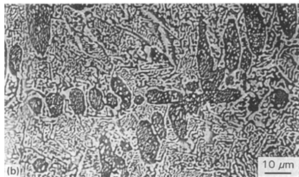
Figure 7 Room-temperature modifications of the eutectic tin-bismuth alloy: (a) 3 hours after casting, (b) 3 days after casting, (c) 3 months after casting.
